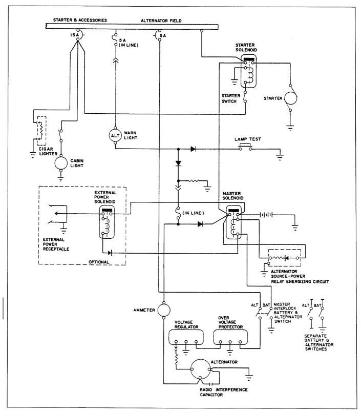
ALTERNATOR AND STARTER SCHEMATIC
